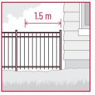
Install non-combustible fencing within 1.5 m of the house (cement fiber, metal, chain link or stone).
