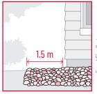
Install non-combustible ground surfaces within 1.5 m of the house (mineral soil, rock, concrete or stone).
